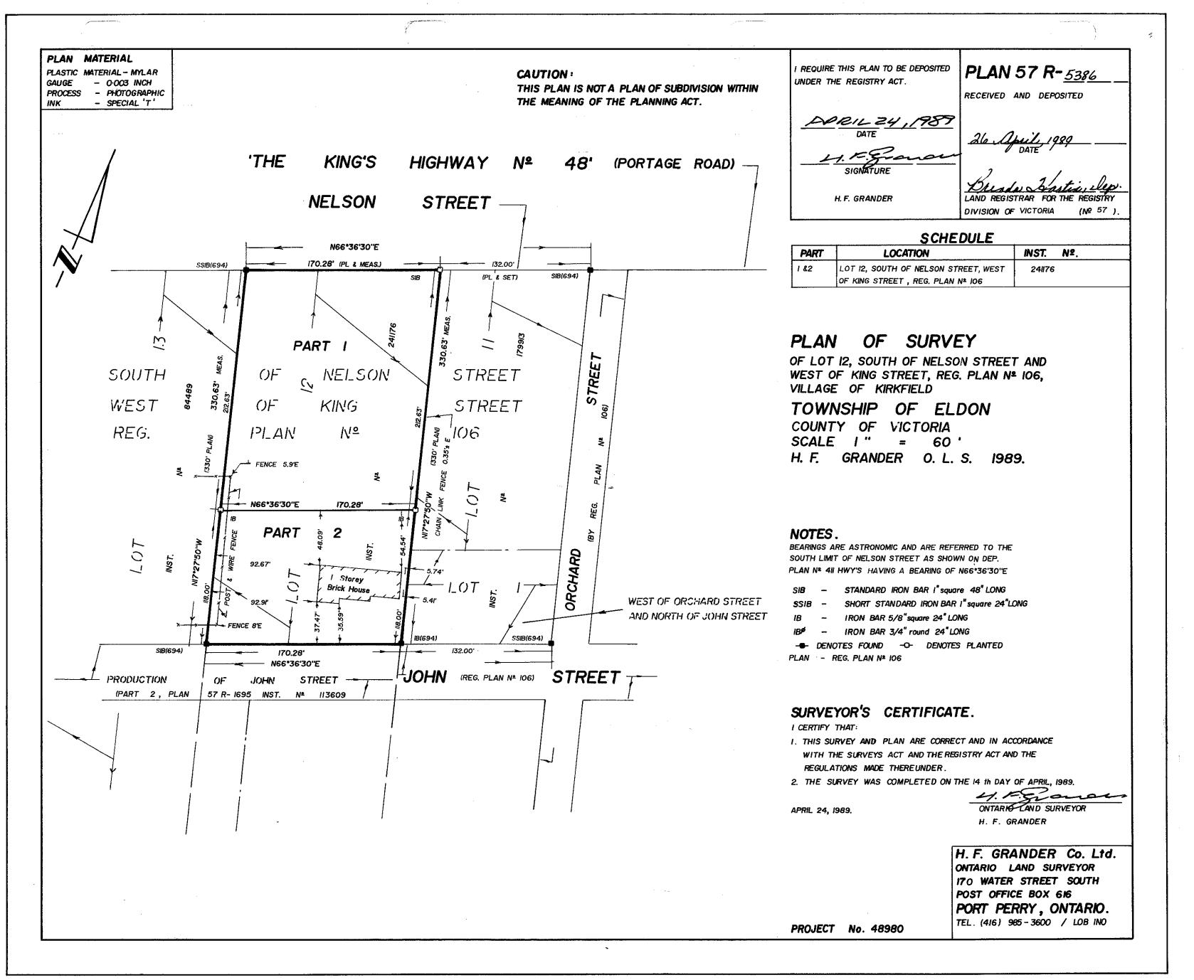
DISTANCES SHOWN ON THIS PLAN ARE IN FEET AND CAN BE CONVERTED TO METRES BY MULTIPLYING BY 0.3048.
